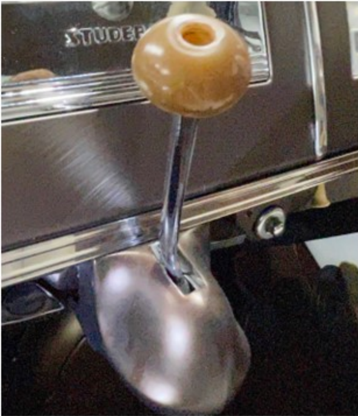
Photo shows the Gearshift on the dash. The Miracle Shift vacuum for manual gearbox was introduced to give a flat floor and comfortable three-across seating. This was a standard option in 1938 only
