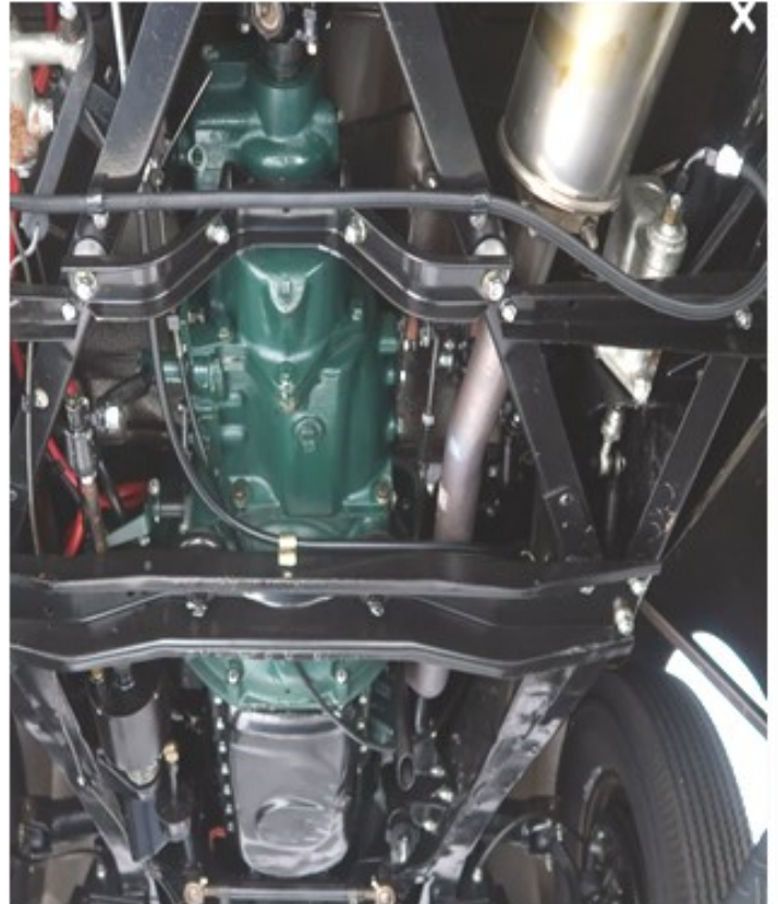
Photo on the right shows the Gearbox, with the vacuum reserve on the left side of the gearbox
